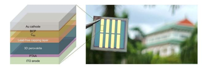
(Left) A diagram showing the different layers of the perovskite solar cell capped with the zinc-based capping material fabricated by the researchers. (Right) The dotted green rectangle indicates the active region of the perovskite solar cell that captures sunlight and converts it to electricity. Credit: NTU Singapore.
