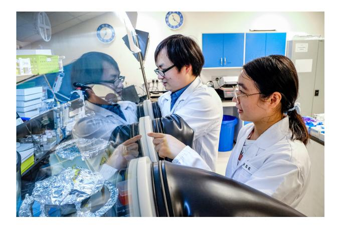
To fabricate the zinc-based capping layer, the researchers dissolved the chemicals and coated the solution onto the perovskite layer in a glovebox. The glovebox protects the perovskite from oxygen and moisture in the environment before it is coated. Credit: NTU Singapore.
